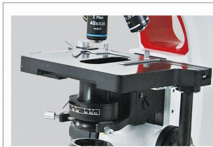
Double-layer mechanical stage, with double slide clips
