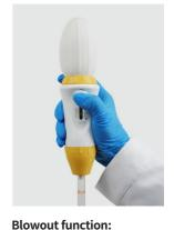
When it is necessary to blow out the liquid, when the concave surface reaches the nozzle, press the blow out ball.
