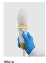
The filling rate can be adjusted continuously with the help of the operating rod.
